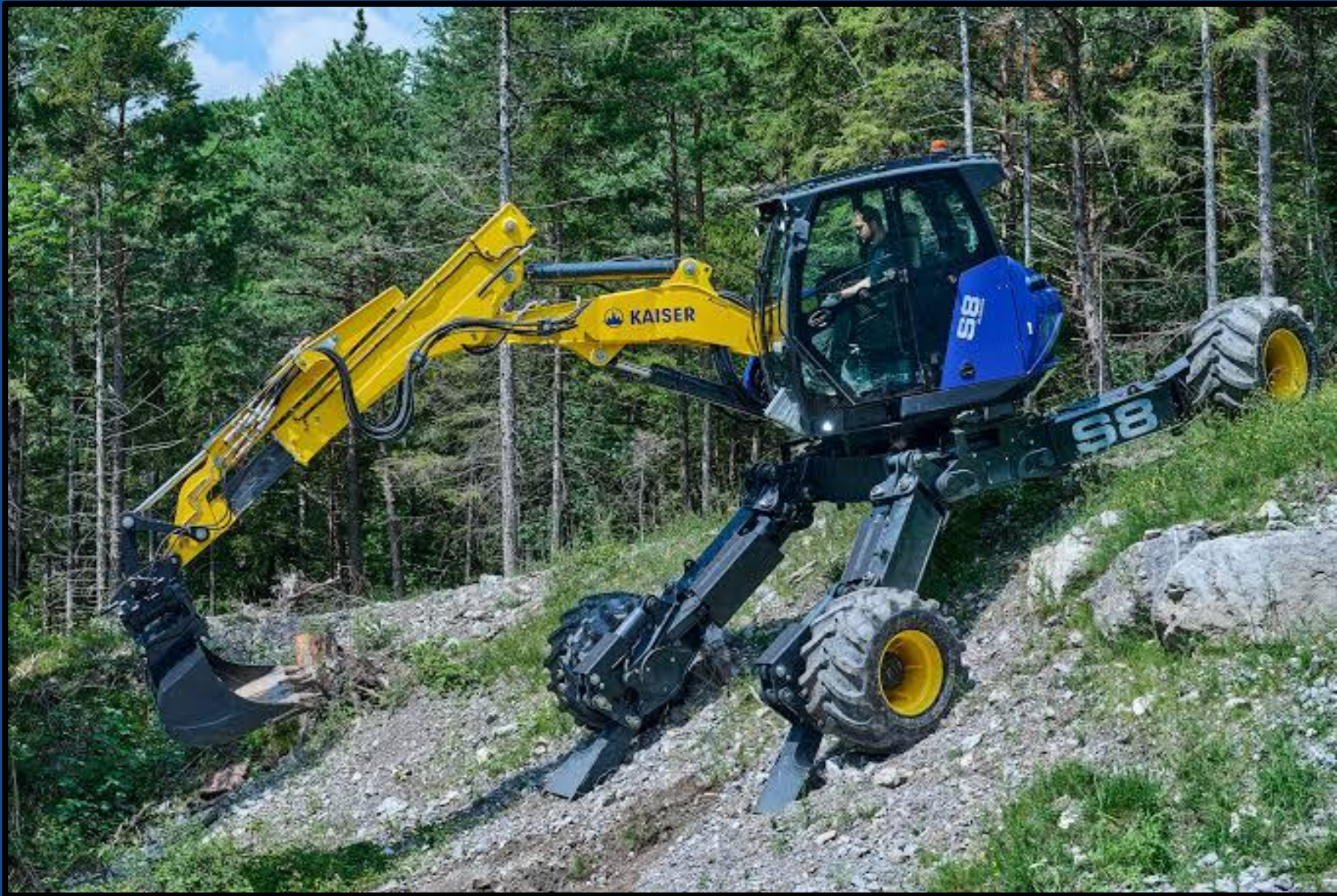
Kaiser S8 Gator Walking/Telescoping Excavator
